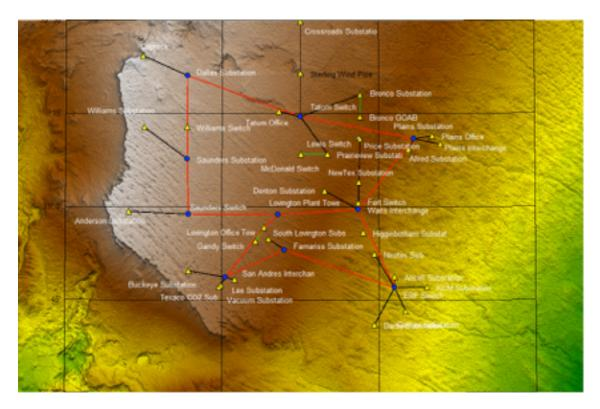
JTS was hired to formulate a solution for a highly reliable system with little to no downtime, alleviating key issues faced, both today and in the future. LCEC identified 36 sites of key importance for communication for which a ring topology solution was identified, connecting 11 hub sites in a ring formation with the remaining 25 sites being connected via spur links.
